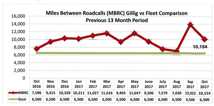
MBRC is a performance gauge of maintenance quality, fleet age, and condition; an increase in MBRC is a positive indicator. As defined by the Federal Transit Administration, a road-call is the practice of dispatching a service vehicle to repair or retrieve a vehicle on the road. There are two types of road-calls; Type I and Type II. A Type I road-call is a major mechanical failure
